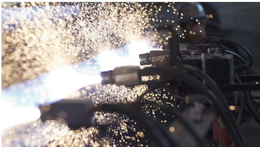
A section of drillpipe undergoes a thermal spray treatment to create protective and friction-reducing wear bands. Source: WhiteHorse Technology.
