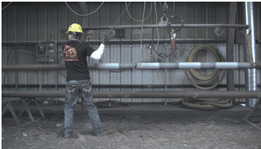
A worker moving a treated drillpipe with four raised wear bands. Source: WhiteHorse Technologies.
